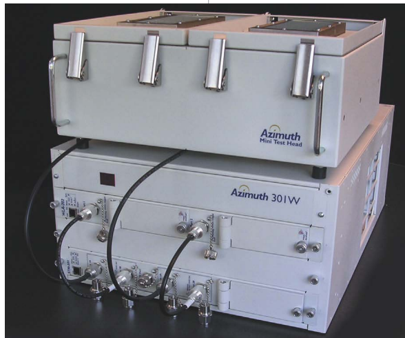
The W-Series modular desktop WiFi-test system is the first to offer fully automated testing of WiFi phones' roaming parameters.
