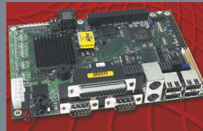
The new Gecko single-board computer in the EPIC form factor fits space-constrained applications with restricted cooling.
